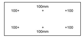
The average velocity must be more than 0.5 m/sec. We recommend commissioning to 0.55 m/sec. Adjust the fan speed as below. Record the velocity measurements in a commissioning report. Conduct a smoke test (AS/NZS 2243.8) and record the observations.
